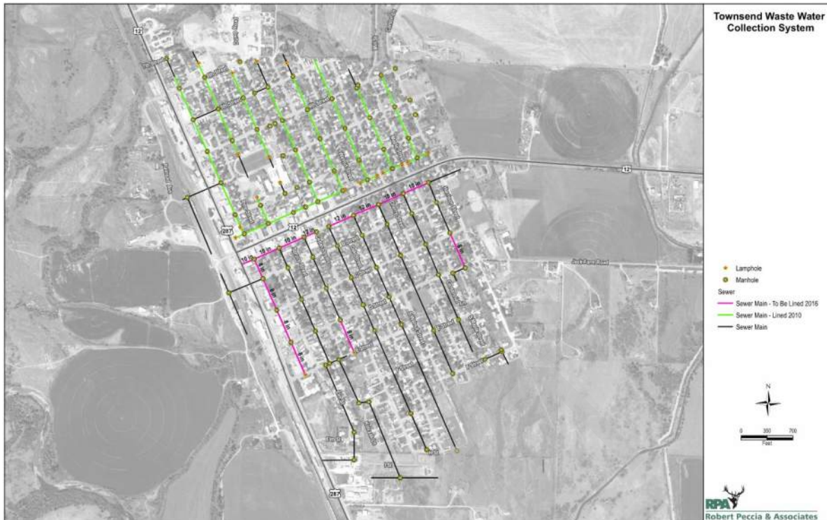
Figure 2. Townsend Wastewater System Map
